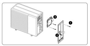
2 Remove 2 screws and pull the plate to the left.
