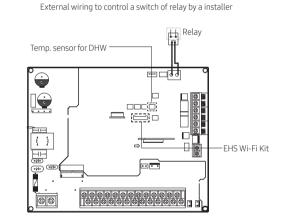
Connecting a temp. sensor wire into DHW
