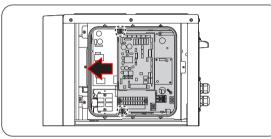
**3** If the plate is rotated to where the hook is, it will be fixed to the hook.
