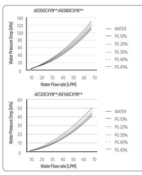
Changing Glycol concentration can cause the pressure drop of the system and it can lead to make flow rate slow.
