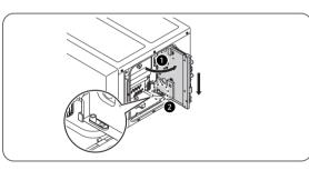
4 Insert the cables at the rear of the unit, and route them through the factory mounted cable sleeves into the switch box.
