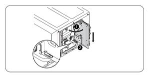
Insert the cables at the rear of the unit, and route them through the factory mounted cable sleeves into the switch box.
