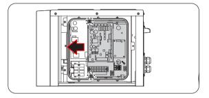
**3** If the plate is rotated to where the hook is, it will be fixed to the hook.
