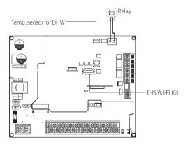
Connecting a temp. sensor wire into DHW
